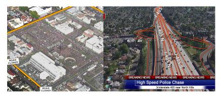
SHOTOVER's next generation augmented reality mapping software, overlays critical geo-referenced information on top of live video. In the aircraft or the control room, operators can interact with the live airborne video and have full control over what is shown on the broadcast feed.
