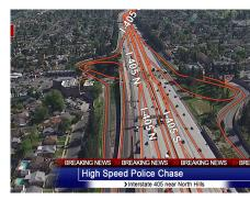
SHOTOVER's next generation augmented reality mapping software, overlays critical geo-referenced information on top of live video. In the aircraft or the control room, operators can interact with the live airborne video and have full control over what is shown on the broadcast feed.
