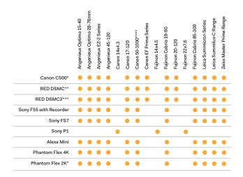
\*The standard G1 configuration includes everything necessary to integrate the above camera and lens combinations with the exception of the Canon C500 and Phantom Flex 2K. The open platform design of the G1 allows for the integration of new cameras and lenses as they come to market. Please note cameras and lenses not included.
