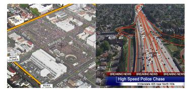
SHOTOVER's advanced AR mapping software overlays geo-referenced data on top of live video, empowering operators in aircraft or control rooms to interact and control broadcast feed content.
